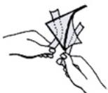
Note: Separate a corner of the 'window film' and liner with 2 small pieces of adhesive tape on either side of the product.
