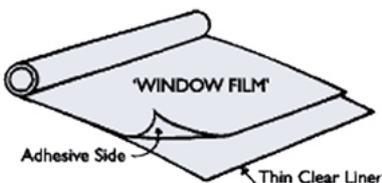
1. Adhesive surface is protected between 'window film' and liner.
