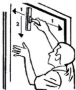
1. Spray the film with the slip solution to give slip for the squeegee.
