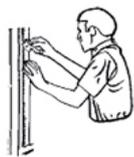
1. Using a straight edge (should have about 1/8" thickness), place it on end at the edge of the window.
